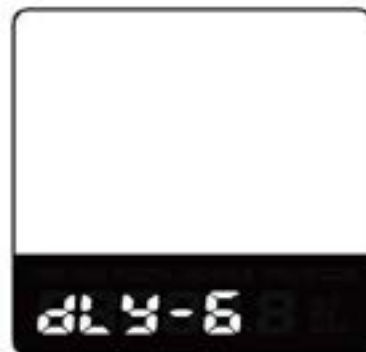
Interface of Battery Power Delay Time Setting
